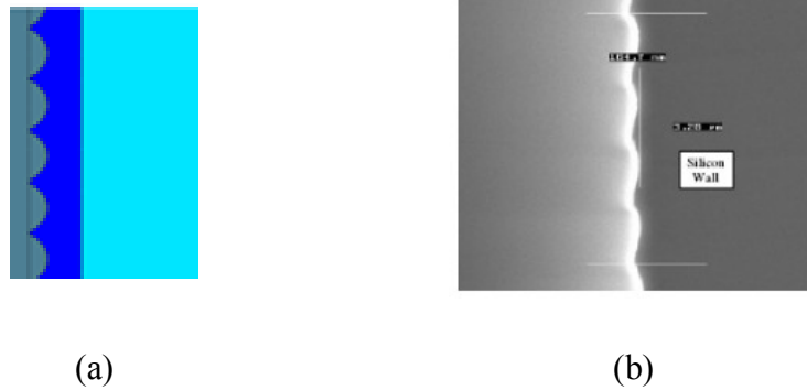
Figure 39: Structure of VJ with sidewalls scalloping. TCAD model (a); SEM image (b)
